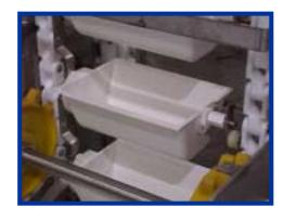
The plastic chain is unique to Gough Econ bucket elevators. It has no rollers and runs on a plastic track. Because of this design, the chain is completely washable and needs no lubrication.
