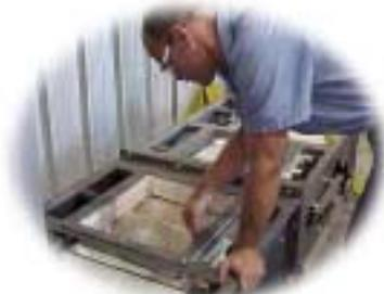
*Main sprockets are checked for proper alignment.*
