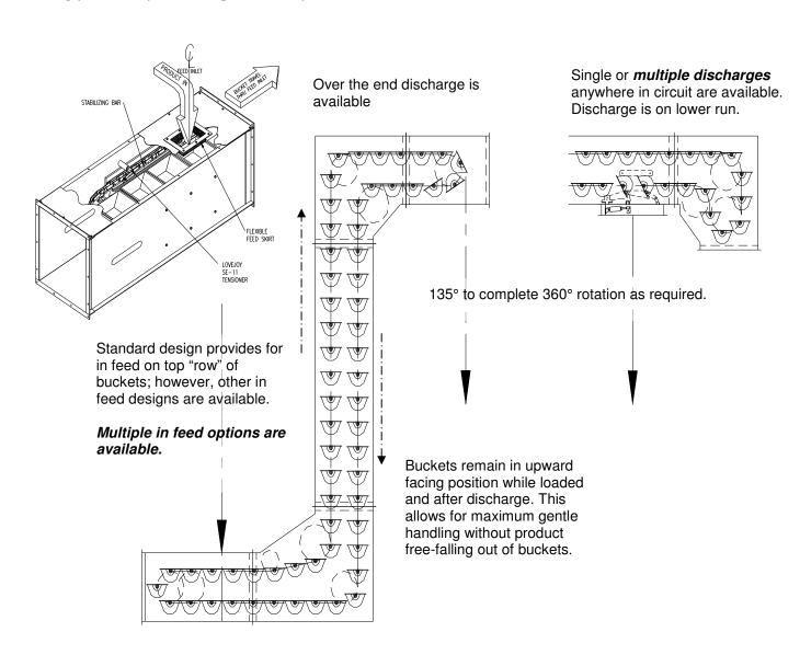
Buckets overlap when in the horizontal position to insure that there is no product spillage during loading of product into buckets.
